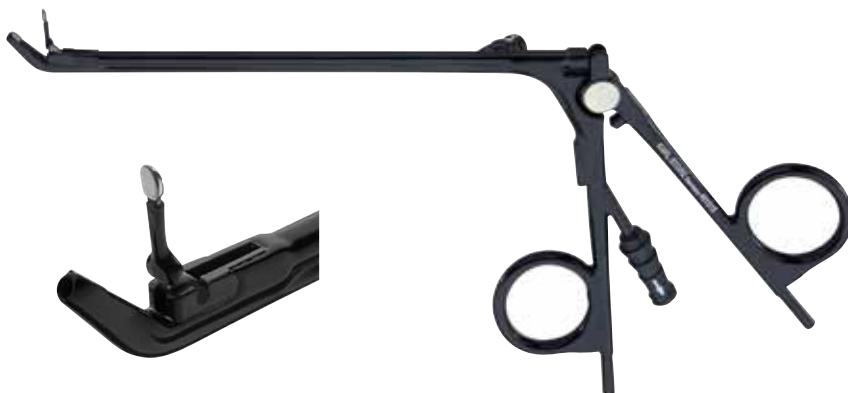
461015 STAMMBERGER Bipolar Suction Forceps , 45° upturned, with suction channel, for bipolar coagulation in paranasal areas, working length 12.5 cm, for use with bipolar high frequency cable 847002 E or 847002 A/M/V
