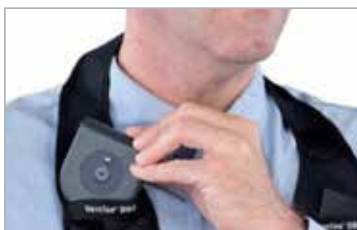
2. Place the Charger Within the Charging Collar
