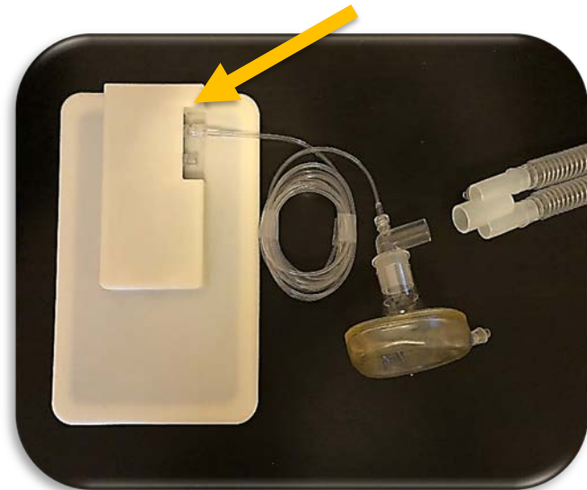
Standard anesthesia equipment connected to the breath sensor port on the custom tablet case
